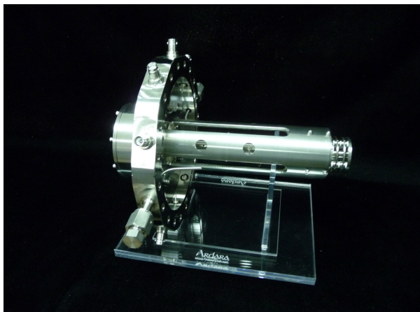
Figure 2. 9 mm quadrupole mounted to a radial flange with extraction optics and Faraday detection.
