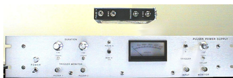
Pulse Power Supply with 5,000 volt bias, 400 volt swing, with Pulser (above).
