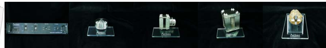
Q-TOF with 9 mm Quadrupole, Rectilinear Collision Cell / Ion Trap, with Orthogonal Extraction Reflectron TOF
