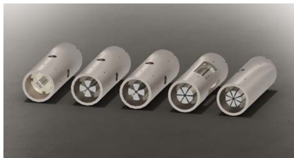
Figure 1. An array of 4mm inscribed diameter ion guides: quadrupole, wide rectilinear quadrupole, narrow rectilinear quadrupole, hexapole, and octopole.
